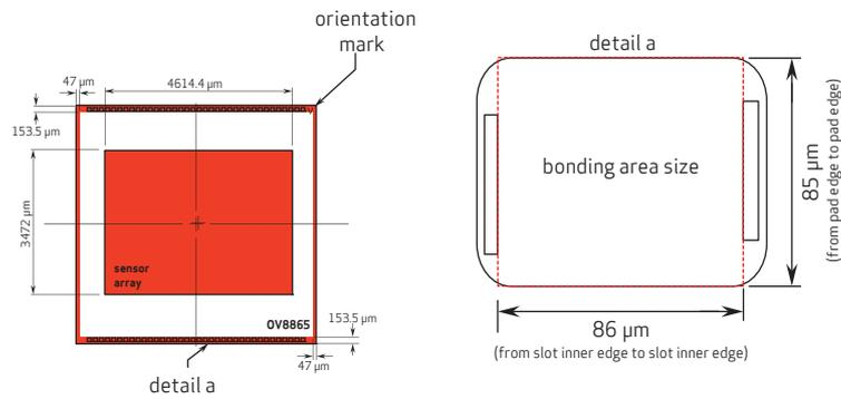
**note 1** bonding outside the defined bonding area is prohibited, it may potentially induce reliability issues or functionality failure
