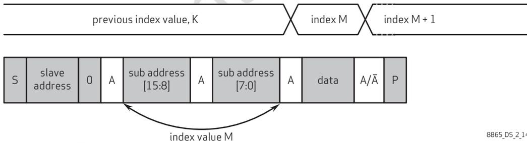
The sequential write is illustrated in **figure 2-15**. The slave automatically increments the sub-address after each data byte. The sequential write operation is terminated with stop condition from the master.
