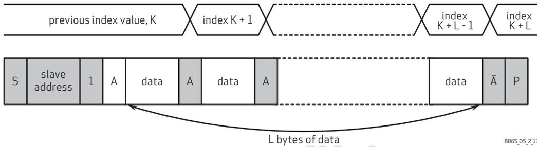
The write operation to a random location is illustrated in **figure 2-14**. The master issues a write operation to the slave, sets the sub-address and data correspondingly after the slave has acknowledged. The write operation is terminated with a stop condition from the master.
