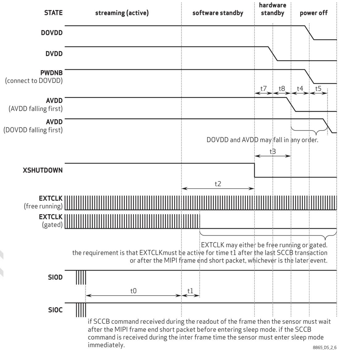
figure 2-7 power down sequence (case 2)
